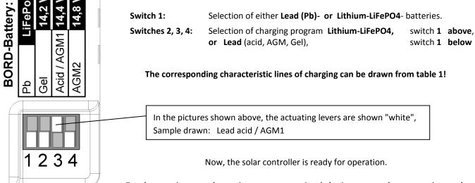
Further actions at the unit are not required during normal automatic mode.
