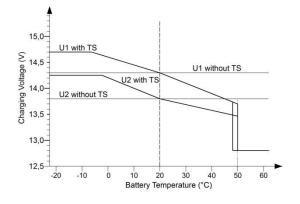
**LiFePO4 Batteries:** Characteristic Line LiFePO4 IU1oU2.
